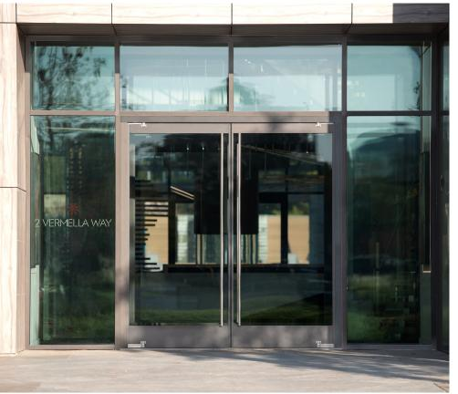
Ellison balanced doors are built to outlast traditional commercial doors and provide a lifetime of easy, trouble-free operation. In addition, balanced doors pivot at two-thirds width, an attribute that more evenly distributes the door's weight, reduces opening force, and relieves air pressure at both sides of the door frame.
